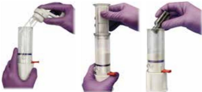
4. Replace top and attach vacuum hose to the vacuum port. (Optional)
