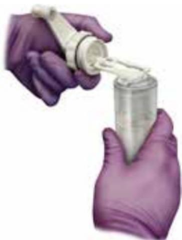
7. Remove red tab and rotate white base counterclockwise to expose syringe port.
