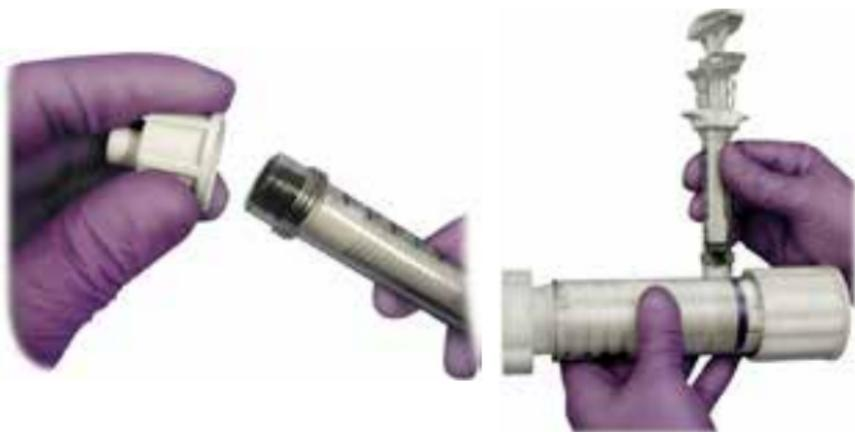
10. While holding mixer on its side, continue rotating/advancing extruder until syringe is full. Disconnect syringe and reconnect syringe cap.
