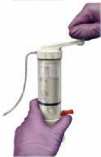
6. Disconnect vacuum hose (if connected), remove top, and scrape excess.
