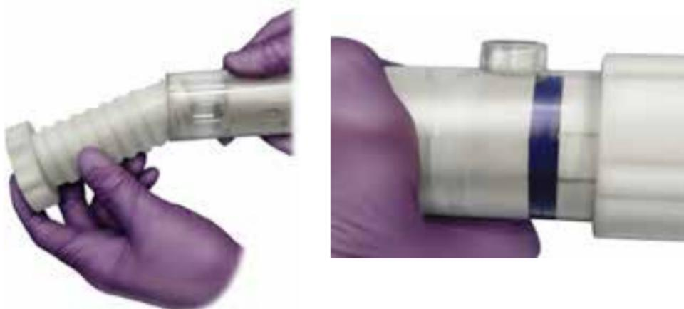
8. Press fit syringe barrel in vertical orientation. While gripping the clear chamber continue rotating/advancing extruder until syringe is filled.
