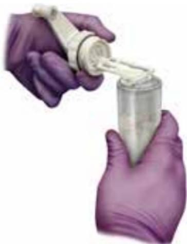
6. Remove red tab and rotate white base counterclockwise to expose syringe port.
