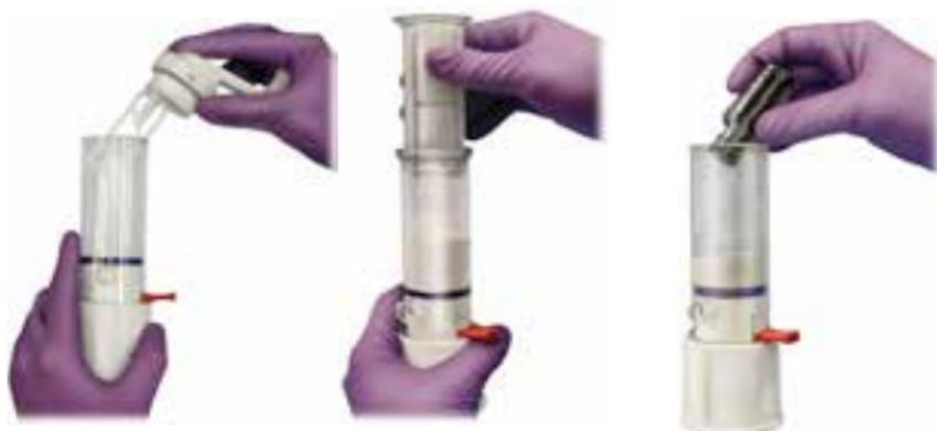
3. Replace top and attach vacuum hose to the vacuum port. (Optional)
