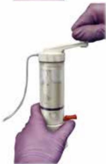
5. Disconnect vacuum hose (if connected), remove top, and scrape excess.
